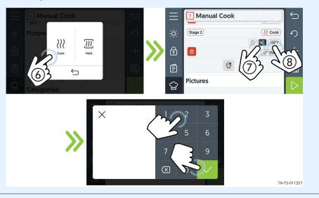
5. **Set** the desired temperature of the cavity. To do so, **touch** the cook temperature **(9)**. **Enter** a cook temperature using the number pad. **Touch** the check mark.
