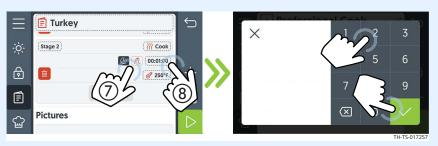
8. **Touch** the chamber temperature set-point icon **(9)**. **Enter** the chamber temperature set-point using the key pad. **Touch** the check mark.
