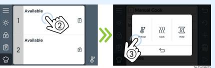
3. **Touch** the preheat temperature **4**). **Enter** a preheat temperature using the number pad. **Touch** the check mark.
