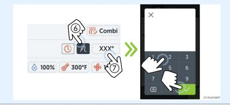
6. **Touch** the cooking temperature icon **(8)**. **Enter** the cooking temperature using the key pad.
