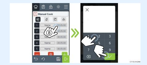
7. **Touch** the cooking time (9) for pan 2. **Enter** the cooking time using the key pad. **Touch** the check mark.
