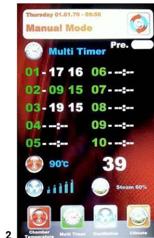
**Fig. 1** – Set the desired timers (max 59 minutes each touching the corresponding number icon, confirming each value pressing again the corresponding icon or the icon of another timer, or using
