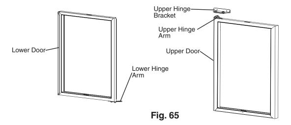
19) While supporting the upper door and upper hinge bracket, place the upper door onto the upper center hinge pin on the center hinge bracket in the closed position, then secure the upper hinge bracket to the cabinet. See Fig. 66. NOTICE! Be sure to reuse the bracket screws for mounting the bracket as the bracket screws are 5×12 and filler screws are 5×10.
