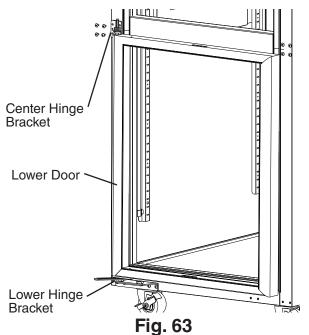
18) Rotate the lower door (making it the upper door) 180 degrees. Rotate the lower hinge bracket 180 degrees. Confirm the thrust washer is in place on the door, then place the new upper hinge bracket onto the upper door pin. See Fig. 65.
