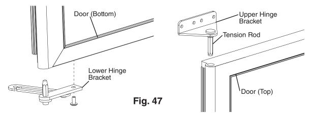
17) Place the door on the lower hinge bracket in the closed position, then secure the upper hinge bracket to the cabinet. See Fig. 48.
