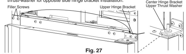
4) Rotate the upper hinge bracket 180 degrees counter clockwise. See Fig. 28. Next, remove the spring cartridge screw and washer, then remove the upper hinge bracket and thrust washers (2). Set the door aside. Retain the upper hinge bracket thrust washers for opposite side hinge bracket installation.
