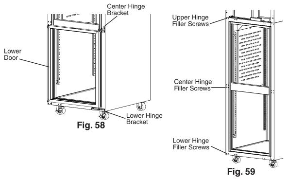
12) Rotate the upper hinge bracket 180 degrees, then place and secure it in the new lower hinge bracket position. See Fig. 60. **NOTICE!** Be sure to reuse the bracket screws for mounting the bracket as the bracket screws are 5×12 and filler screws are 5×10.
