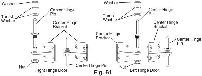
14) Rotate the upper door (making it the lower door) 180 degrees and place the center hinge bracket lower pin into the top of the now lower door. See Fig. 62
