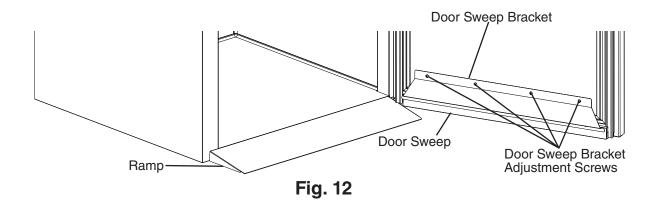
5) Adjust the door sweep so that the door sweep touches the ramp when the door is closed. See Fig. 13. Once in its correct position, tighten the door sweep bracket adjustment screws.
