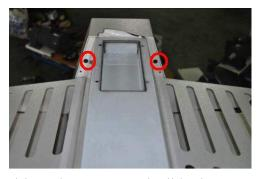
5. Once the (4) Screws holding the Front Panel have been removed, slide the Front Panel away from the Sheeter (use flathead screwdriver if needed to gently pry the Panel apart from the frame). Be cautious while removing the Front Panel as there are wire connections that go to the Mico Switches.
