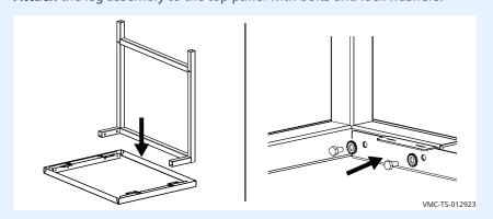
Install the second leg assembly into the top panel.
