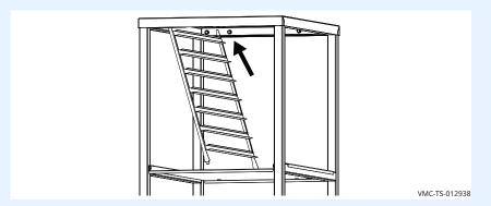
9. **Rotate** the side rack and lower it into the slots on the shelf.
