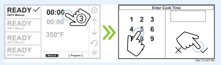
3. **Touch** the temperature setting **4**). **Enter** the cooking temperature using the number pad. **Touch** the check mark.
