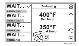
The screen displays the chamber's actual temperature and its set temperature. Selecting different chambers displays information on their respective temperatures.
