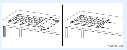
4. **Install** jet plates 5029095 in the lower section of each chamber with the part number facing up. **Install** jet plates 5030451 in the upper section of each chamber with the part number facing down.
