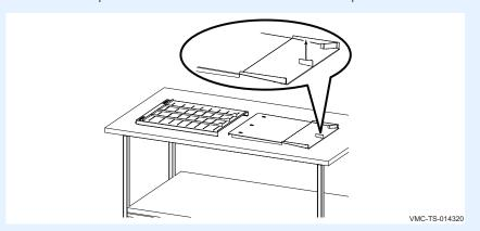
3. **Insert** the inner panel into the outer panel. **Push** the inner panel into the outer panel until it is fully inserted.
