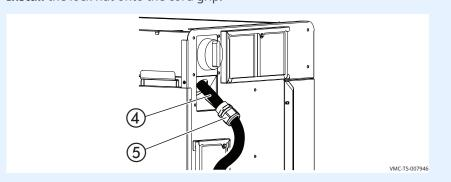
7. **Connect** the supply cord to the appropriate terminals (L1, L2, L3, etc.) in accordance with local codes and regulations.
