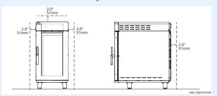
2. **Move** the oven to the installation location and onto the final resting surface.
