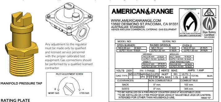
The information on the rating plate defines the model, serial number, gas type (Natural Gas or ULPG), operating pressures and burner BTU ratings. Keep this information for future reference. It is essential for proper identification of the unit when requesting additional information or factory support.
