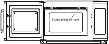
2.The left hand grasp the microwave, right thumb to press the arrow directions and forced to push back. And the left thumb hard pressed upward at the same time. put the right of oil blockage into the buckle of the feont plate.
