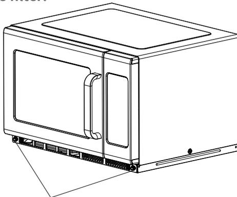
To restall,align the base plate mounting holes,
