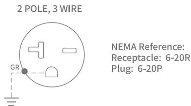
Consult a qualified electrician or serviceman if the grounding instructions are not completely understood, or if doubt exists as to whether the appliance is properly grounded. If it is necessary to use an extension cord, use only a 3-wire extension cord that has a 3-blade grounded plug, and 3-slot receptacle that will accept the plug on the appliance. The marked rating of the extension cord shall be equal to or greater than the electrical rating of the appliance.
