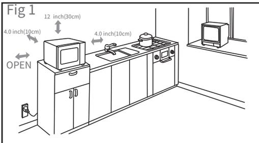
A 4.0-inch spacing should be kept between the appliance and right and back walls, and a 12-inch spacing kept on the top. Never dismantle the appliance's feet, nor block the air intake and exhaust opening. The left side must be open.
