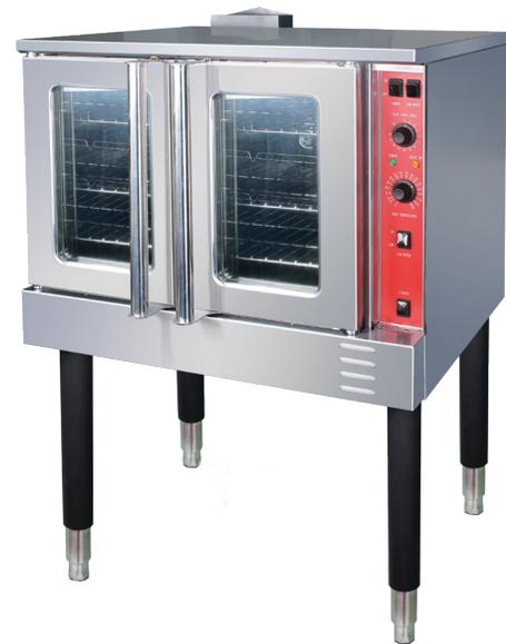
Recommended incoming gas pressure: Natural 6" W/C, LP12" W/C. The internal pressure regulator is factory set for proper operating pressure of 4.0" W/C for Natural and 1.-." W/C for LP. The operation pressure should be checked and verified upon installation.
