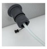
Now screw together the individual components of the splash protection cover.
