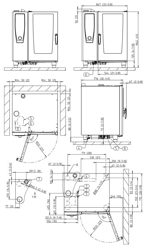
1. Common water supply (cold water) "Single" water connection as shipped 2. Water supply cold water / condensate "Split" water connection 3. Water supply cold / Treated "Split" water connection 4. Water drain 5. Electrical connection wire entrance 6. Chassis Ground connection 7. Steam Vent pipe DN 2 3/8" / 60 mm minimum distance 2" / 50 mmLeft side clearance 20" recommended for servicing of unit without the ability to move unit while connected. Measurements in mm (inch)
