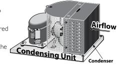
4. If you have a significant dirt build up you can blow out the condenser with compressed air.
