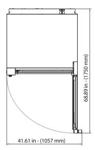
\* Oven must be installed a minimum of 19.7" (500 mm) from any significant source of heat and/or grease (for example: fryers, burners, kettles, open flames, etc.)
