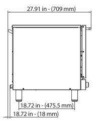
\* Oven must be installed a minimum of 19.7" (500 mm) from any significant source of heat and/or grease (for example: fryers, burners, kettles, open flames, etc.)
