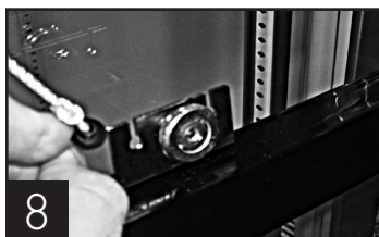
Door roller bracket with nylon cord.
