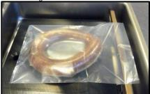
If the product is small, use the included insert plates to reduce empty space in the chamber. This will reduce the cycle time.
