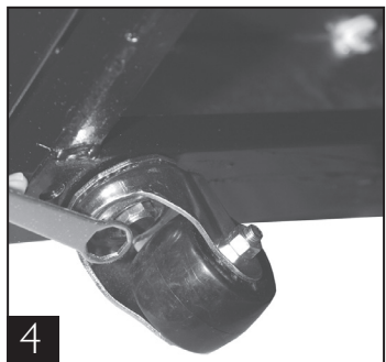
Tighten castor in position with castor wrench.
