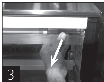
Squeeze lampshield and rotate out.
