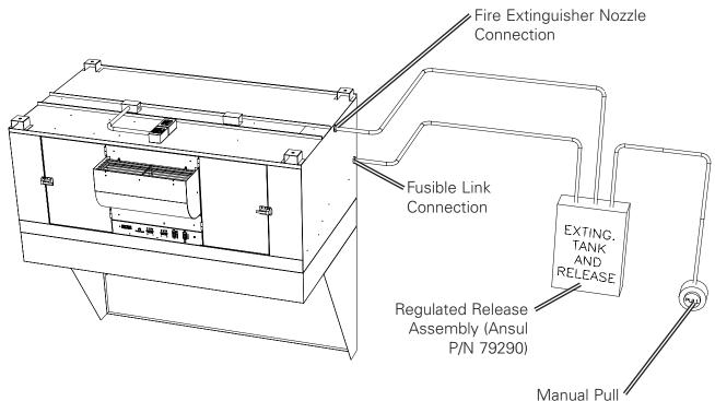
Note -System may be located and connected on the left or right of the hood.
