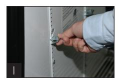
Shelf clips are installed with the front clip lower than the rear clip. This will allow the shelf to tilt forward.
