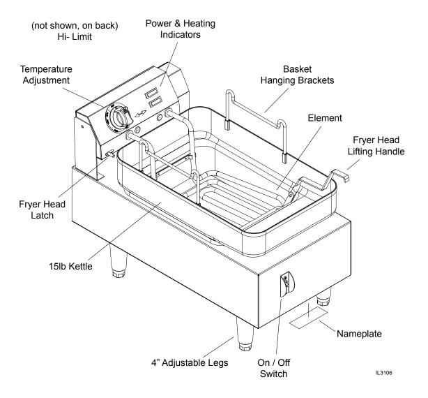
Fig. 1 Countertop Electric Fryer (shown with the fryer head in the down position)
