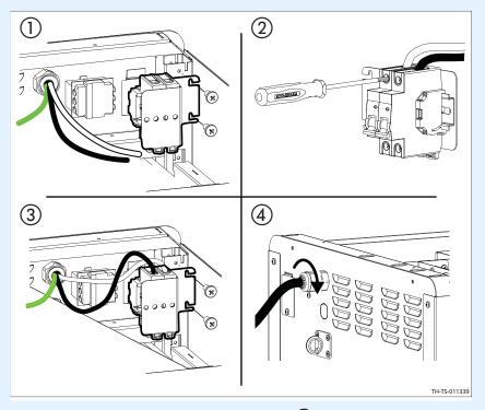
$\textbf{Re-install} \text{ the circuit breakers with the screws } \ensuremath{\mathfrak{3}}.$
