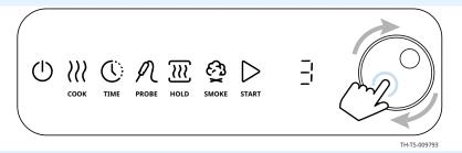
5. On double cavity ovens only, **turn** the knob to select the cavity to save the recipe to (top, bottom, or both).
