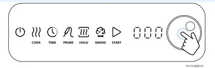
3. **Turn** the knob until the control displays "Stor".
