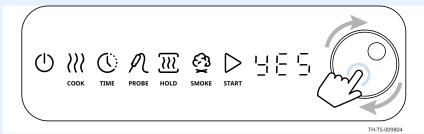
The START icon will display. The light around the knob will flash. The display will go blank for several seconds. The interface board (IB) software version displays. The control board (CB) software version displays. Record this number.
