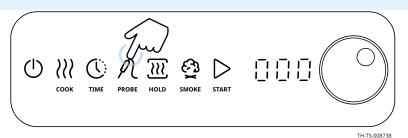
5. **Turn** the knob to set the probe alarm temperature.
